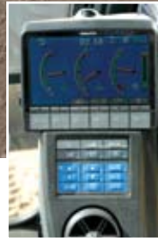
Both the PC220LC-8 and PC200LC-8 have five working modes, including a new attachment mode. The units also feature a large, new color monitor with an "eco-gauge" to further improve fuel efficiency.
