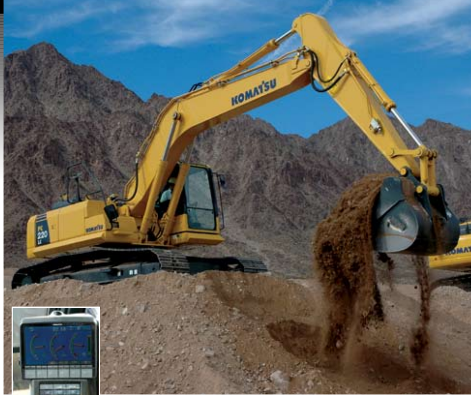
Both the PC220LC-8 and PC200LC-8 have five working modes, including a new attachment mode. The units also feature a large, new color monitor with an "eco-gauge" to further improve fuel efficiency.
