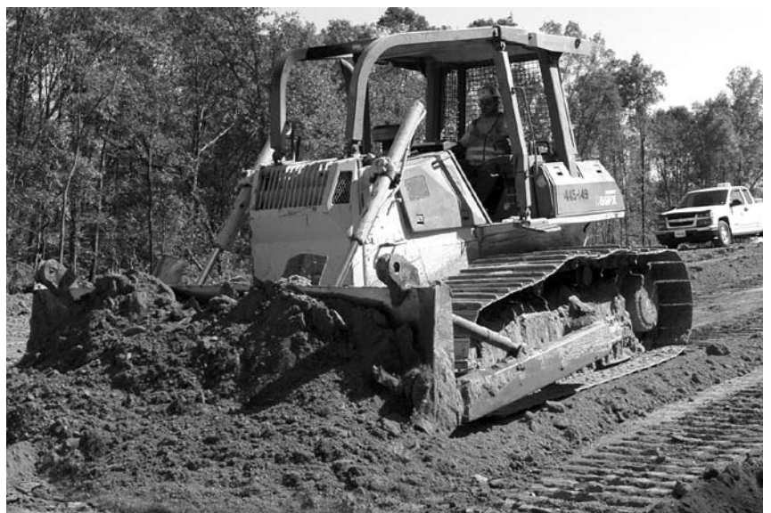
A Hill Bros. operator uses a Komatsu PC300LC-7 excavator to set pipe on a highway project near Memphis. The company, which owns a vast number of Komatsu machines, used a D65 dozer for backfilling operations.
