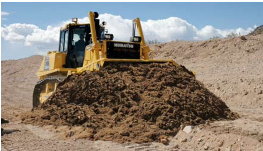
The Sigma Dozer blade is designed to promote rolling of material and to keep it from spilling around the sides.
