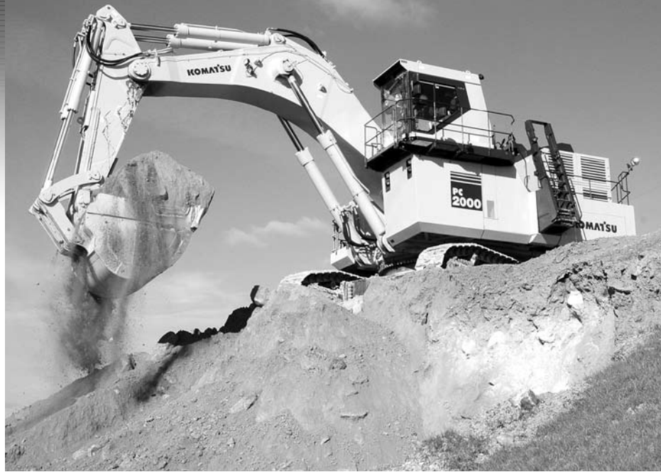
The 956-horsepower PC2000-8 (above) is a new machine that replaces the PC1800 in the Komatsu excavator lineup. Similarly, the new PC800LC-8 (below), has more horsepower and greater stability than the PC750 it replaces.
