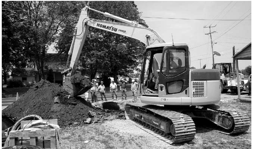
Byard Construction's tight-tail-swing Komatsu PC138 excavator can work in tight spaces where its PC300 and PC200s can't. "It digs well," said Owner Jim Byard. "I'm tickled to death with that little machine and how it works in every tight spot we get into."
