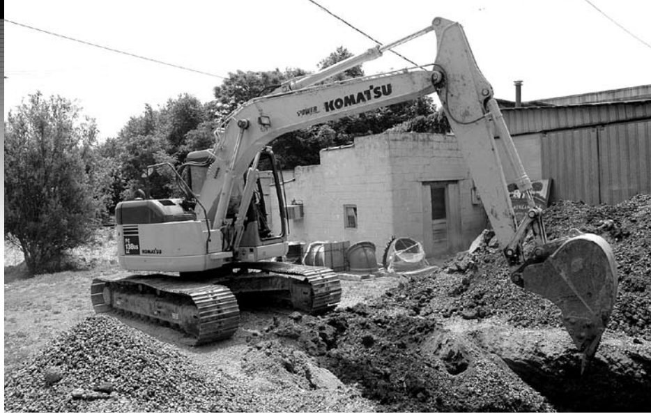
Byard Construction's tight-tail-swing Komatsu PC138 excavator can work in tight spaces where its PC300 and PC200s can't. "It digs well," said Owner Jim Byard. "I'm tickled to death with that little machine and how it works in every tight spot we get into."
