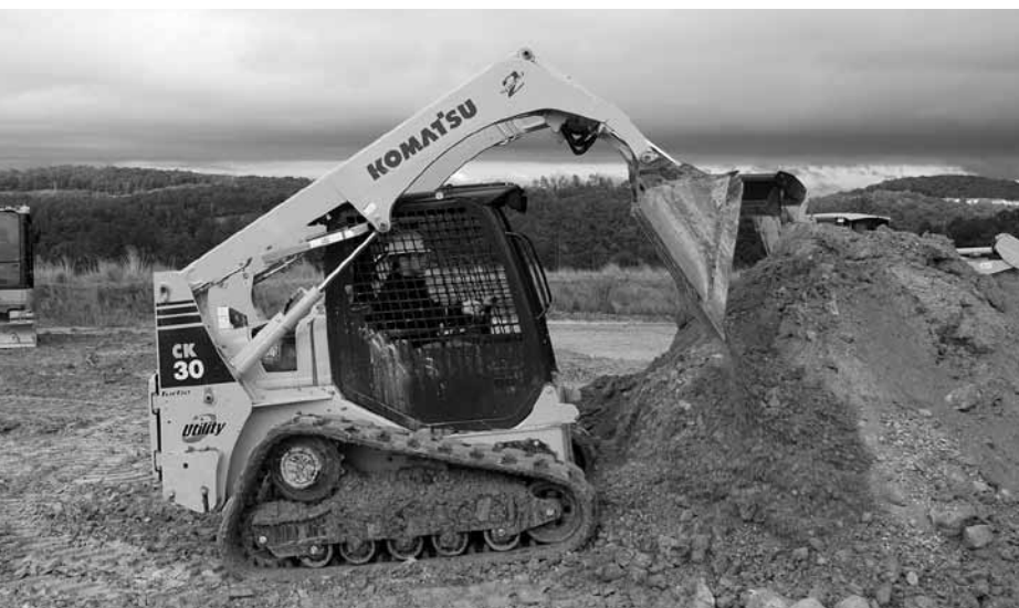
Utility machines, such as the CK30 compact track loader, were required to meet Tier 4 emission standards in 2008. Tier 4 is on the horizon for 175 horsepower and up machines in 2011 and 75 to 175 horsepower must be Tier 4 in 2012.
