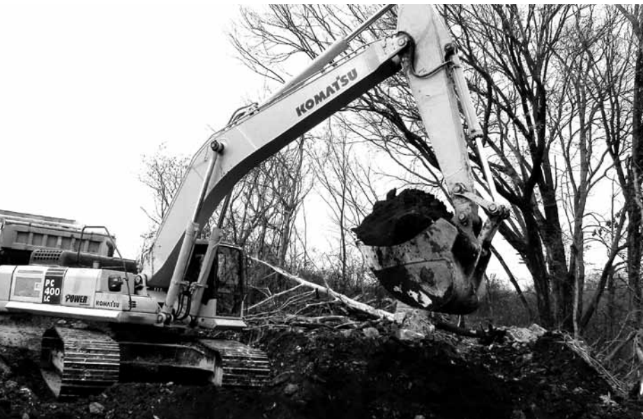
Equipment Operations Manager Cameron Druyor uses KOMTRAX to monitor Rogers Group's Komatsu equipment, including this PC400LC-7 that's removing overburden at REOStone Quarry in Nashville.
