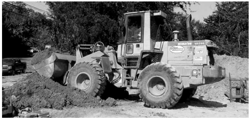
Hurst Excavating runs a variety of Komatsu equipment, including this WA250 wheel loader used to backfill a trench on a project in Knoxville.
