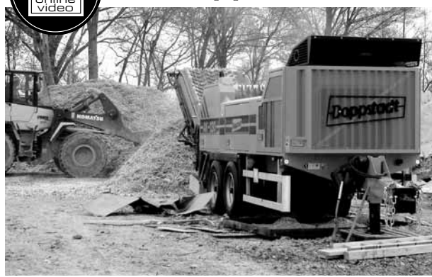
Wright's recently added this Doppstadt AK 230 grinder to process pallets into mulch. "It tears through a pile rather quickly without any worry of binding up," said Owner Nick Wright.
