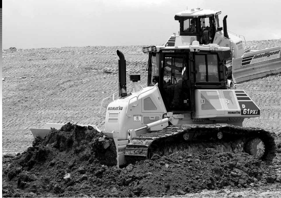
Komatsu introduced its new D61i-23 intelligent Machine Control dozers with integrated grade-control technology that provides automated blade control from rough-cut to finish grading. According to Komatsu's Ed Powers, the machines have received rave reviews.
