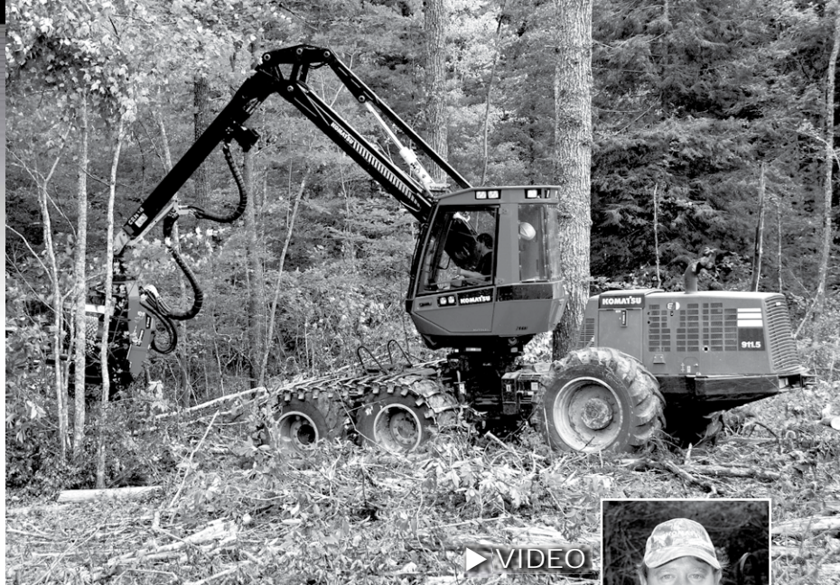
Operator Roger Linville fells, delimits and cuts with a Komatsu 911.5 wheeled harvester equipped with a dangle head processor. "It's quicker and gets around easier than what we used before," said Linville.
