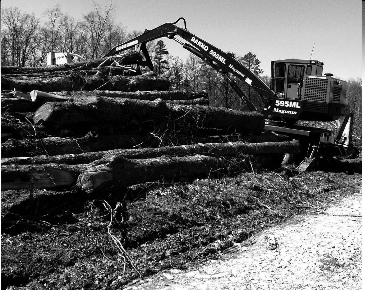
Bill Clark Logging uses a Barko 595ML Magnum knuckleboom loader to delimb and cut logs to length. "We wanted something that would handle heavy wood, and the 595 does that, no problem," said Bill Clark Jr. "It has good power to pick up even the heaviest logs. It definitely speeds up production."
