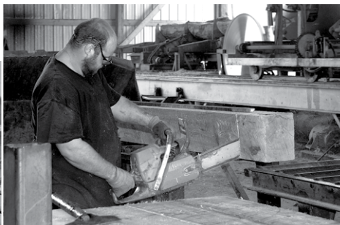
Walnut Creek Timber personnel saw logs into ties, then cut them to length with chain saws.
