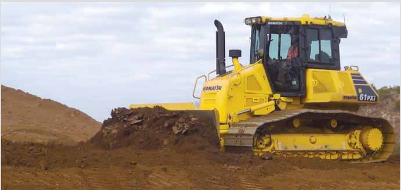
Komatsu introduced its intelligent Machine Control (iMC) dozer line with the D61i-23 about a year ago. It provides automatic blade control from rough-cut to final pass, with an integrated GPS system that eliminates masts and cables.
