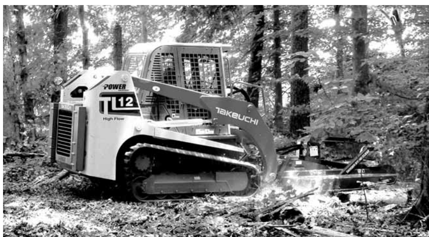
A Takeuchi TL12 compact track loader equipped with a brush cutter attachment was available for demonstration.
