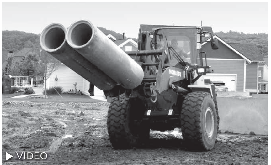
A Carbine & Associates operator moves concrete pipe with a Komatsu WA200PZ wheel loader at the Tollgate Village project.
