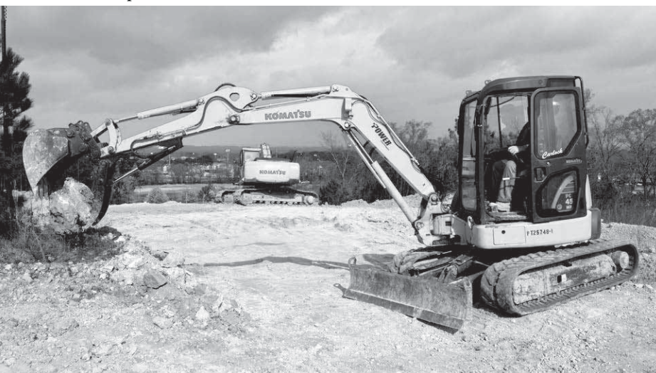
A Carlock Trucking & Construction operator uses a Komatsu PC45MR-3 excavator to clear stumps.
