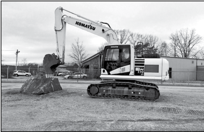
2017 Komatsu PC170LC-10 9'6" stick, 36" bucket, S/N 30549, 1,467 hrs.
