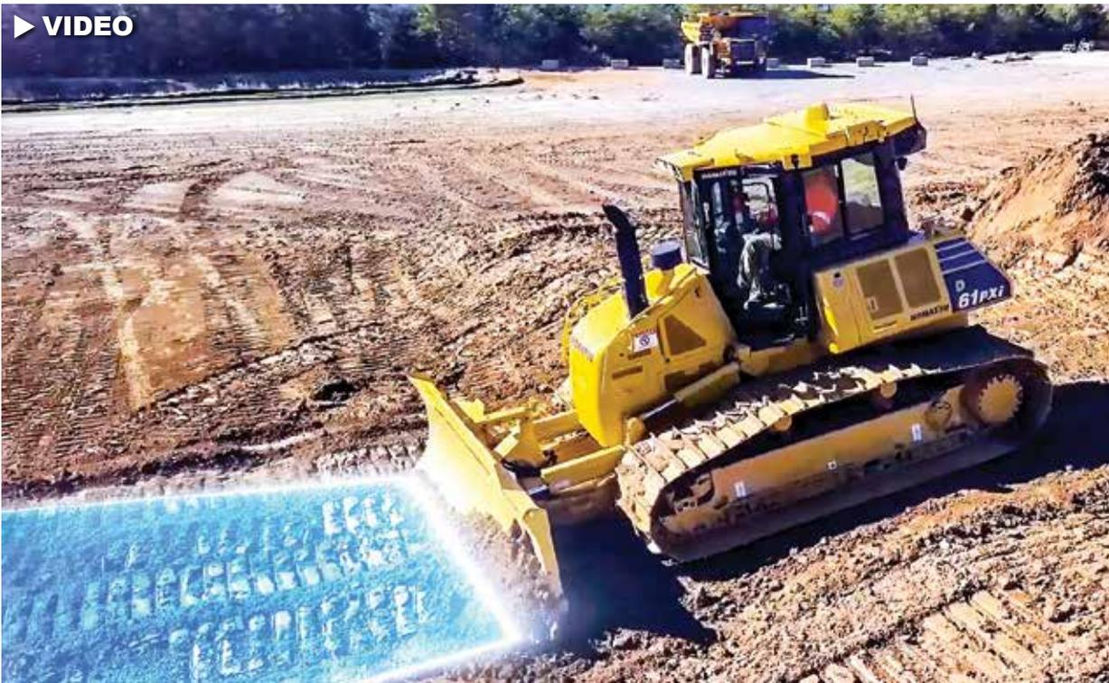
Proactive Dozing Control logic understands what the terrain around the machine looks like and decides whether to cut and carry material, spread or fill with it or whether it should finish grade, just like an experienced operator. The integrated GPS grade control system works from first pass to last to perform everything from auto-stripping to final grading.
