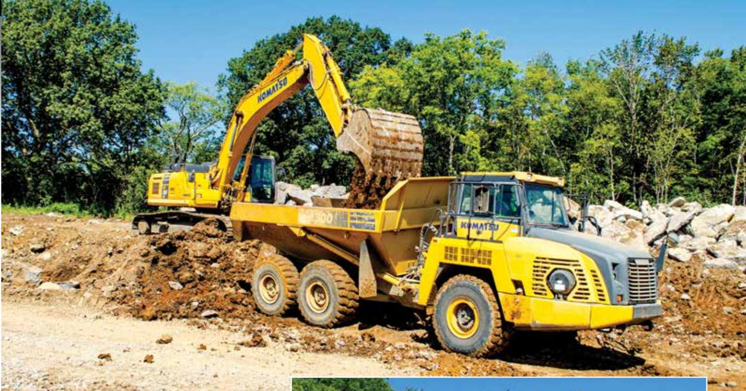
Using a Komatsu *intelligent* Machine Control PC360LCi excavator, a Covenant Constructors operator loads the company's HM300 truck while simultaneously grading a pad at Burkitt Ridge subdivision in Nolensville, Tenn. "It's a lot more efficient," said Project Manager/Estimator Michael Dickson. "With the PC360LCi, he is able to dig and fill the truck while remaining on grade."
