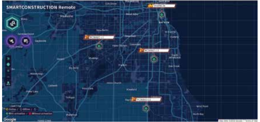
With Smart Construction Remote, contractors can see the site and where their intelligent Machine Control dozers and excavators are working in near real time. Updated design data can be sent directly to the machines from off-site locations via GPS.
