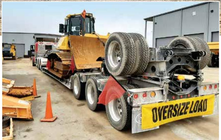
A J&D Specialized Equipment Hauling truck driver prepares to haul a Komatsu D51PX dozer from Power Equipment Company's yard on an Etnyre Blackhawk trailer.
