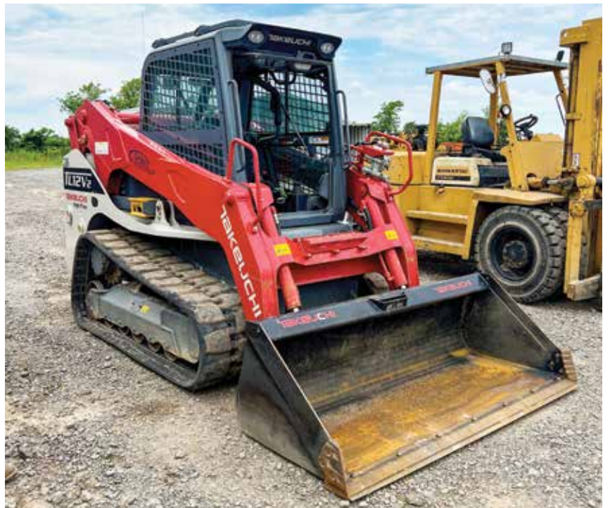
Grace Railroad Contractors' fleet includes a Takeuchi TL12V2 compact track loader. "We use it when we are replacing track for larger railroads or if a derailment causes a track wipeout," said Dustin Grace, president/CEO. "We take the excavators and throw all the steel and cross ties out of the way and use the compact track loader to knock it flat, so we can put down new track. You can pull up to a pile and shove through it like a dozer."
