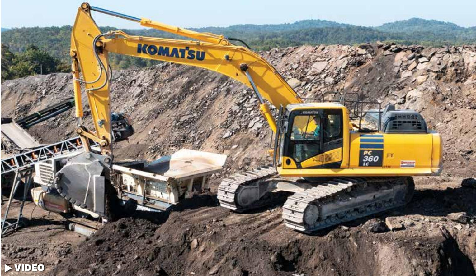
An operator moves asphalt millings with a Komatsu PC360LC-11 excavator at Duracap's recycling operation. "It's an all-around good size for handling stockpiles," said Duracap General Manager Camden Guyton. "It has the right amount of power to load material into the crusher."
