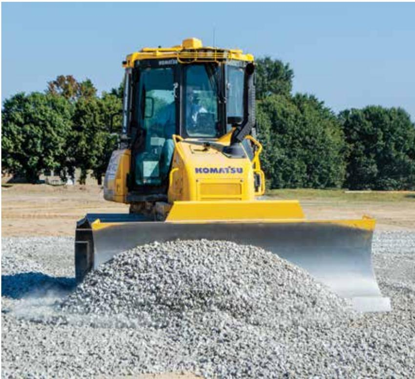
An operator pushes rock with a Komatsu D39PXi-24 iMC dozer. "The D39 was the perfect size because it is so adaptable to different-sized projects and allows us to work in a safer way," said FARCO President Taylor Meharg.
