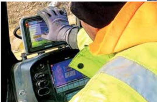
A Tomahawk Construction operator cuts a road in the early stages of a project with a Komatsu D51PXi-24 iMC dozer. "In our experience, nothing works as well as Komatsu," said Project Surveyor Randall Hendra. "With Smart Construction Remote, I'm able to update changes to our models and remotely send them to our GPS-equipped Komatsu machines without having to separately drive to each machine and install the file with a thumb drive."
