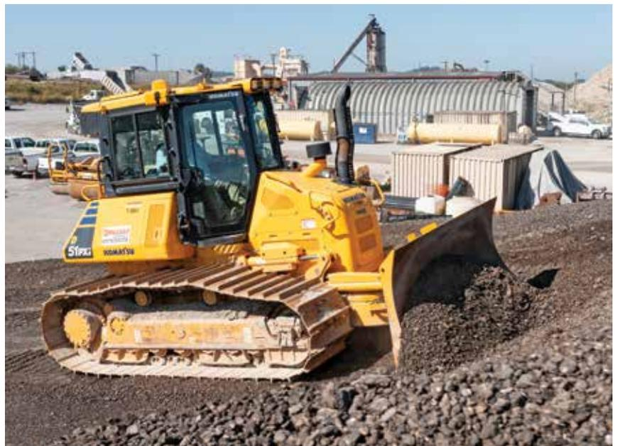
With a Komatsu D51PXi-24 intelligent Machine Control (iMC) dozer, Duracap General Manager Camden Guyton pushes material at an asphalt plant. "The machine is tied in with our GPS layouts and that simplifies our jobs," said Camden. "We invested in the iMC machine to make it a little bit more efficient on that end."
