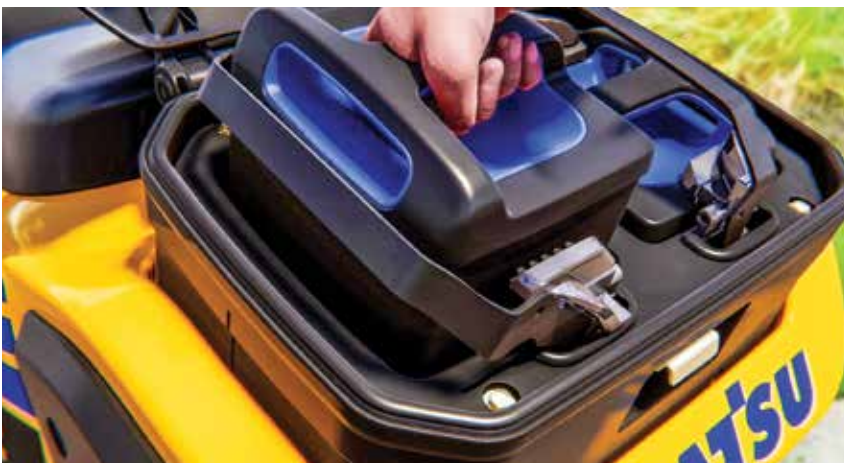
An operator places a battery in an electric Komatsu machine. "While electrification is at the forefront of everyone's mind due to automotive, our equipment on the construction site is often creating that infrastructure for electric automobiles," remarked Andrew Earing, Director of Tracked Products and Service at Komatsu.
