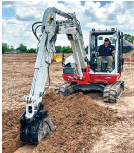
Demo Day attendee John Brewer tests Komatsu's Smart Construction Retrofit on a Takeuchi TB370 compact excavator. "I like the idea that you can put GPS and 3D technology on a small machine," said Brewer. "With Retrofit, you get a series of beeps you can listen to, and it keeps you on grade as you go."
