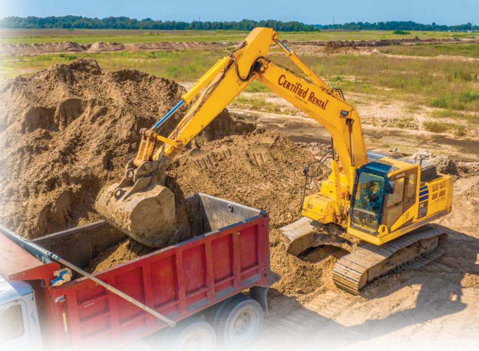
With a Komatsu PC210LC excavator, an operator loads a customer's truck with soil. Typically, 65 to 75 trucks are loaded at Middleton Farms per day.
