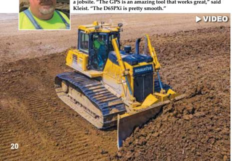
To hit those high production numbers, James Peterson Sons required every bit of the D65PXi's 220-horsepower Tier 4 Final engine and 24.4-ton operating weight. More importantly, it needed that muscle in the correct package. That's why the company selected the PX model, which features wider tracks and a six-way blade.
