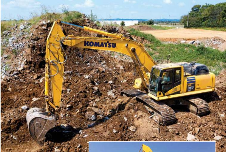
A Floyd & Floyd Contractors operator grades and loads trucks with the company's Komatsu *intelligent* Machine Control PC360LCi-11 excavator at a Mount Pleasant, Tenn., jobsite. "Being able to do both jobs with the PC360LCi is amazing," said Estimator Casey Floyd. "The *intelligent* Machine Control takes so much time out of the equation."
