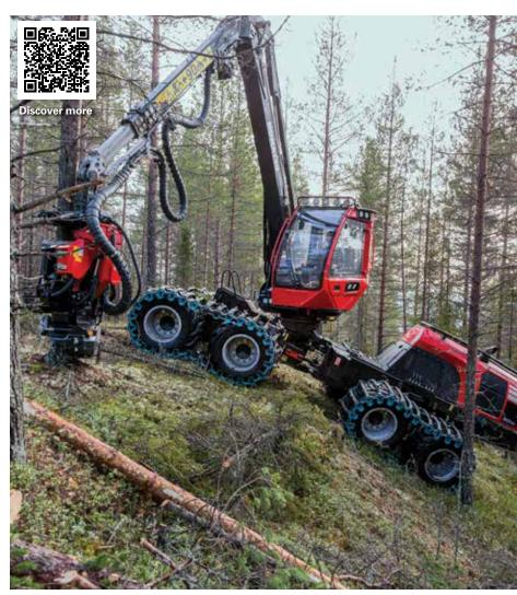
The Komatsu 901XC harvester features a "double Comfort Bogie axle" 8-wheel-drive system designed to tackle steep, uneven, rough and soft terrain. The system generates 12 percent more tractive effort and reduces rear ground pressure compared to the 901 6WD model.
