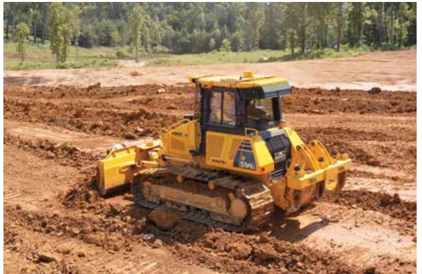
An operator cuts a pad to grade using a Komatsu D51EXi-24 iMC dozer.
