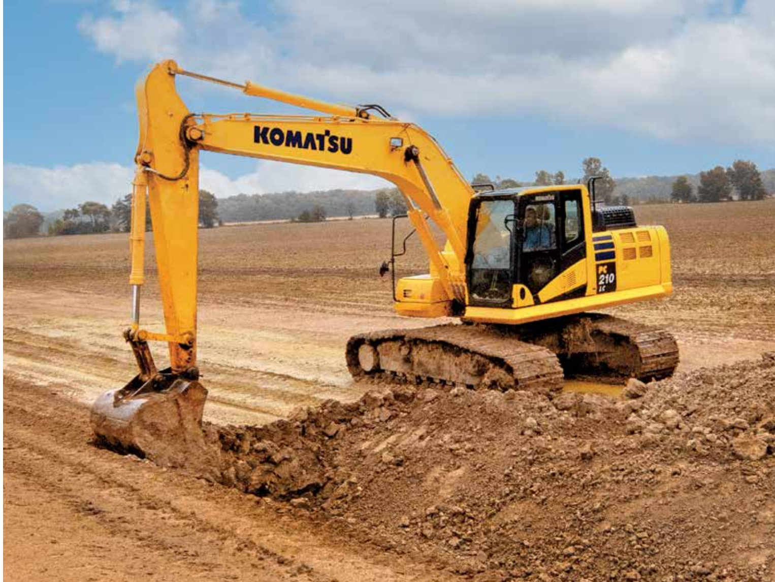
At an Arkansas farm that lost 70 acres of crop, owner Mike Creasey digs an inside re-lift ditch with a pump-off station using a Komatsu PC210LC-11 excavator. "If I'm digging a still water pit and booming up 12 feet with a full load of dirt, the machine doesn't stall out," said Creasey. "I'm able to smoothly transition the digging motion and do it with speed. At the end of a 10-hour day, I'm able to get off the machine without feeling like I've been tossed around."
