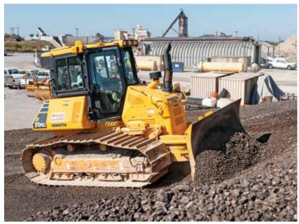
With a Komatsu D51PXi-24 intelligent Machine Control (iMC) dozer, Duracap General Manager Camden Guyton pushes material at an asphalt plant. "The machine is tied in with our GPS layouts and that simplifies our jobs," said Camden. "We invested in the iMC machine to make it a little bit more efficient on that end."
