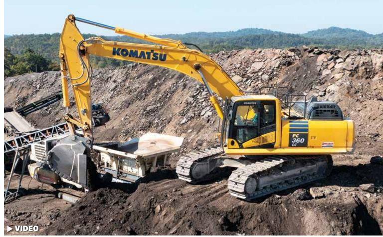
An operator moves asphalt millings with a Komatsu PC360LC-11 excavator at Duracap's recycling operation. "It's an all-around good size for handling stockpiles," said Duracap General Manager Camden Guyton. "It has the right amount of power to load material into the crusher."
