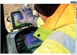
A Tomahawk Construction operator cuts a road in the early stages of a project with a Komatsu D51PXi-24 iMC dozer. "In our experience, nothing works as well as Komatsu," said Project Surveyor Randall Hendra. "With Smart Construction Remote, I'm able to update changes to our models and remotely send them to our GPS-equipped Komatsu machines without having to separately drive to each machine and install the file with a thumb drive."
