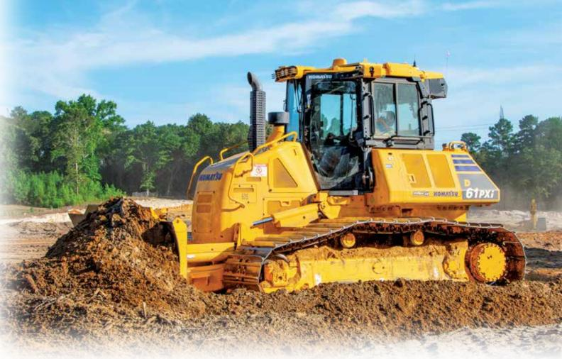
Komatsu's D61i-24 IMC 2.0 dozer is the second generation of the original IMC dozer introduced in 2013. Its features include proactive dozing control, lift layer control, tilt steering control, and quick surface creation.
