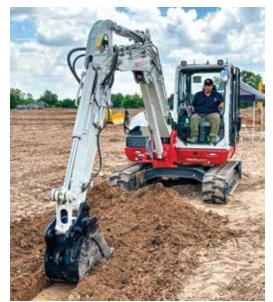
Demo Day attendee John Brewer tests Komatsu's Smart Construction Retrofit on a Takeuchi TB370 compact excavator. "I like the idea that you can put GPS and 3D technology on a small machine," said Brewer. "With Retrofit, you get a series of beeps you can listen to, and it keeps you on grade as you go."
