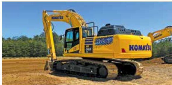
Komatsu's HB365LC-3 hybrid excavator delivers eco-conscious performance as energy is captured during swing and stored in the ultracapacitor.
