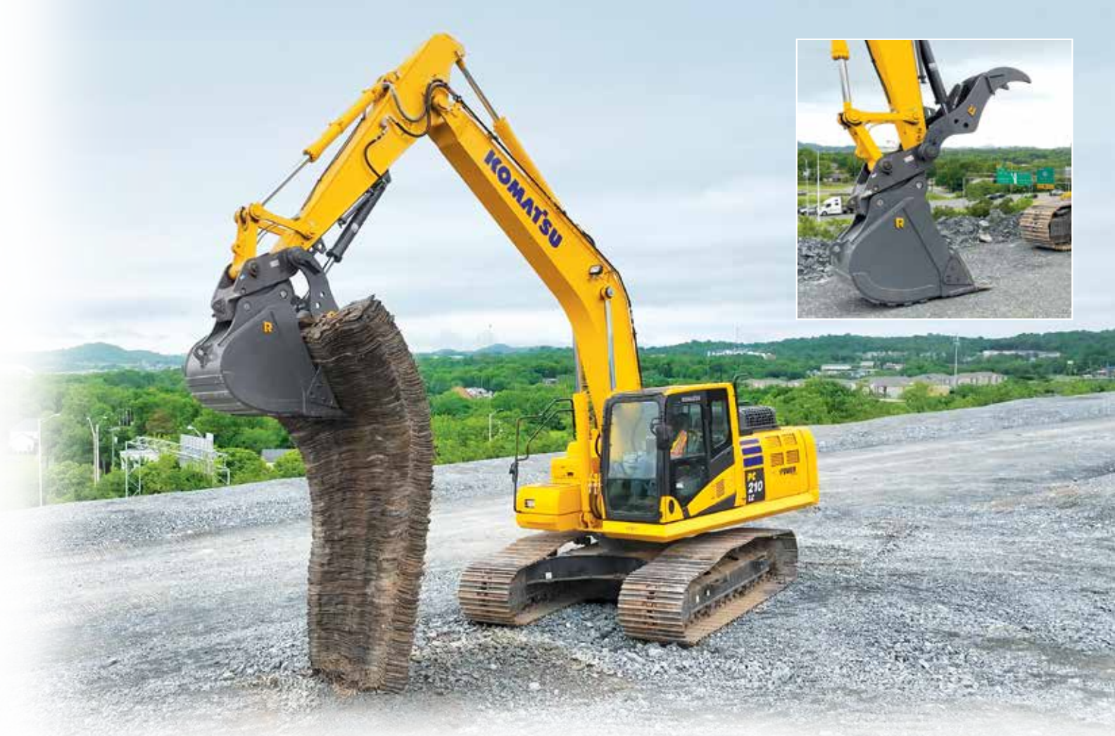
Robert Spickard moves a blast mat with a Komatsu PC210LC-11 excavator outfitted with a hydraulic bucket and thumb.
