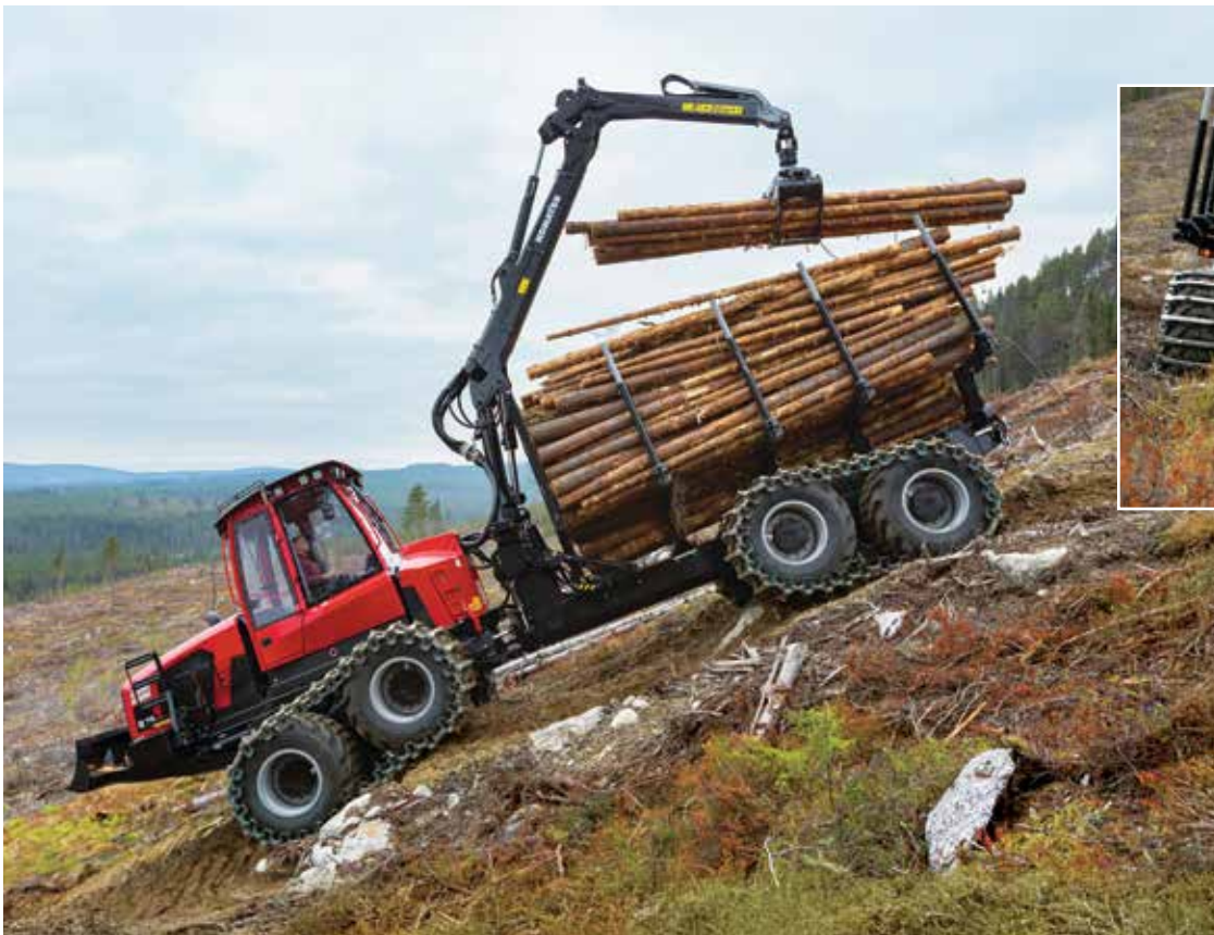
Available as an option on the Komatsu 875 forwarder and the Komatsu 931XC harvester, the Komatsu Traction Aid Winch is a high-quality system that provides extra tractive force and grip to the standard model. It is designed to help the machine navigate even tougher terrain than without the option.
