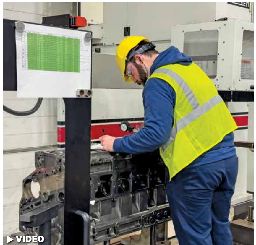
Taking precise measurements to return components to OEM standards is a key step in SRC of Lexington's operations.
