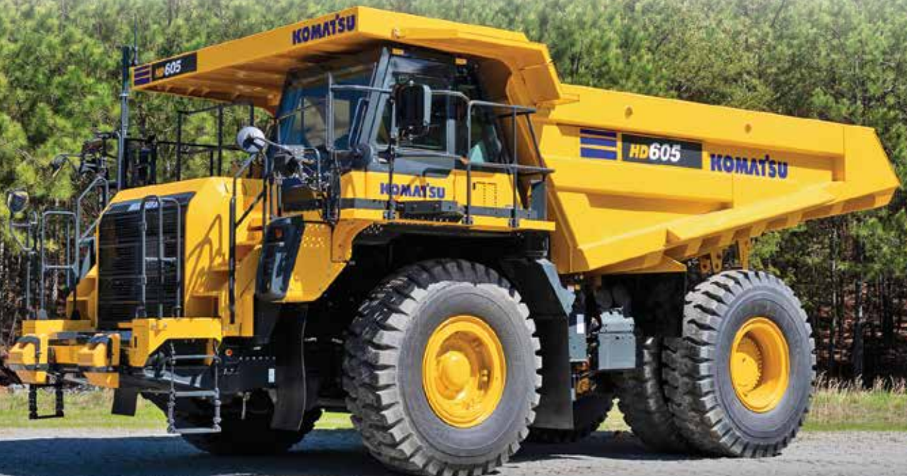
The new Komatsu HD605-10 mechanical haul truck is a 70-ton rigid frame machine designed for reliability and durability.
