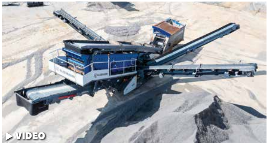
A KLEEMANN MOBISCREEN MS 953i mobile screening plant is used to sort material.
